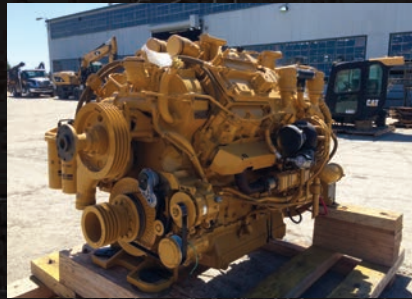
Top to bottom: Peterson's Doug Brecheisen working on Sukut's 5110B onsite; 800 hp C27 engine at the San Leandro shop yard
