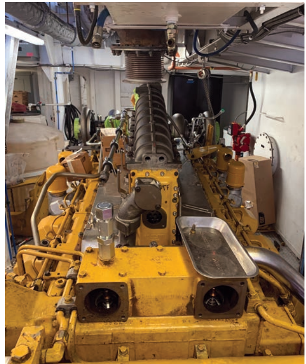
AmNav repower converted two 3516 Tier 2 engines to Tier 3 in 2020
