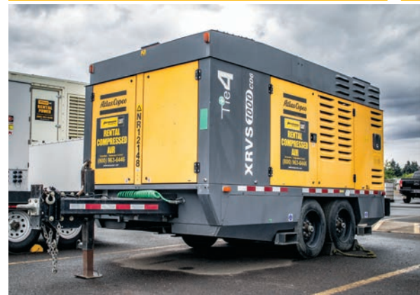
Rental air compressor unit
