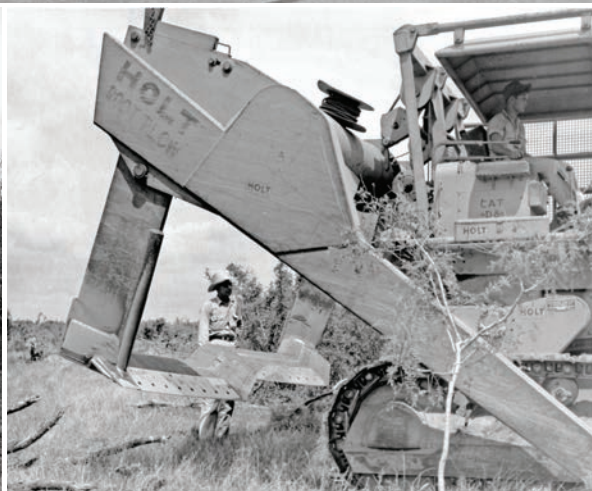
Top/left, clockwise: Hand-scrawled notes for the Holt funnel dozer in the mid-1940s; Holt Funnel Blade attachment on Twin D8 in 1950; King Ranch Twin in transport in 1950; King Ranch Twin w/Holt attachments working in the early 1950s
