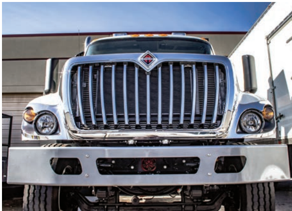
Today's trucks have wider grills to accommodate larger radiators and more complicated engines.
