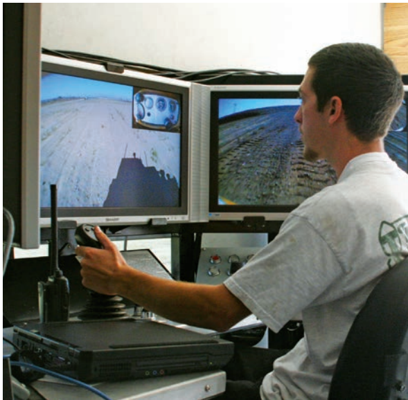
Top to bottom: Armored bomb scraper testing in Pleasanton, California; Virtual cab gives operator control from one mile away.
