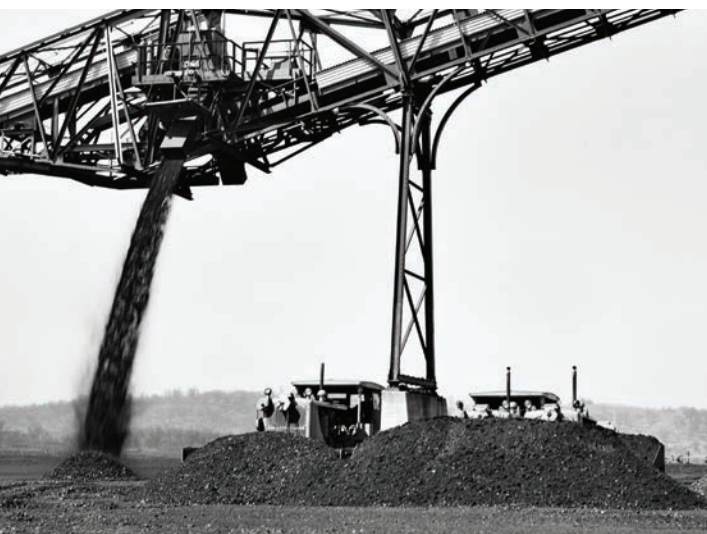
Left to right: Two tractors (twin on the right) pushing coal as it is diverted onto the pile from a conveyor; Tanners Creek Power Plant in Lawrenceburg, IN on the Ohio River in 1992
