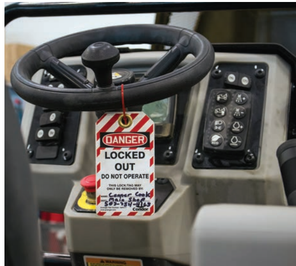
Top to bottom: Roll-up door partially raised, a violation of company safety policy; Machine with lockout tag
