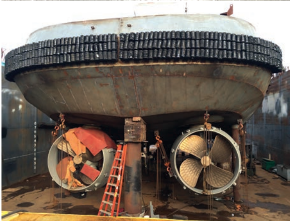
Top to bottom: One of the first Cat Propulsion azimuth thruster systems went into the Dr. Hank Kaplan tug in 2016; Inside vessel; Exterior
