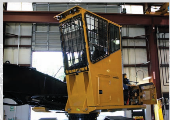
Rear-entry cab installation in shop
