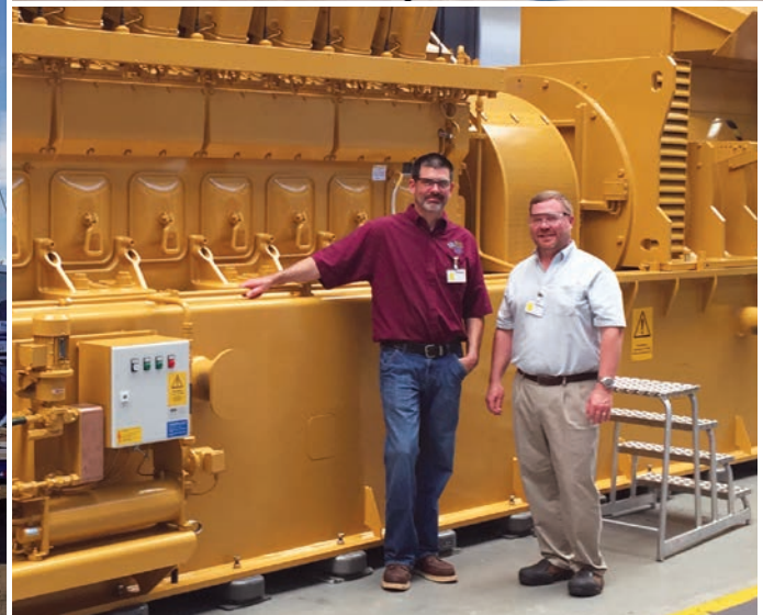
Left, clockwise: City of San Jose cogeneration project; Each of the four CG260-16 engines are 26-ft long, 11-ft high and weighs nearly 60 tons; Marty Hopkins/R with customer at the Cat factory in Mannheim, Germany in 2018
