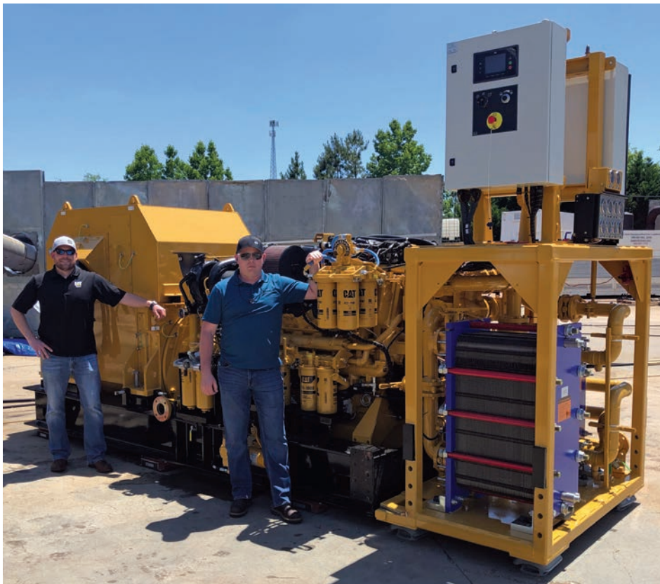
(L-R) Barrett Carpenter and Tyler Raymond/project manager in front of one of the Cat L32 gen-sets for OSU research vessel in 2019
