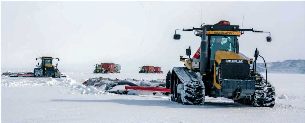
The Traverse departs McMurdo Station on the month-long journey to the South Pole. One tractor can pull 24,000 gallons of fuel in bladders on top of sheets of HMW plastic.
