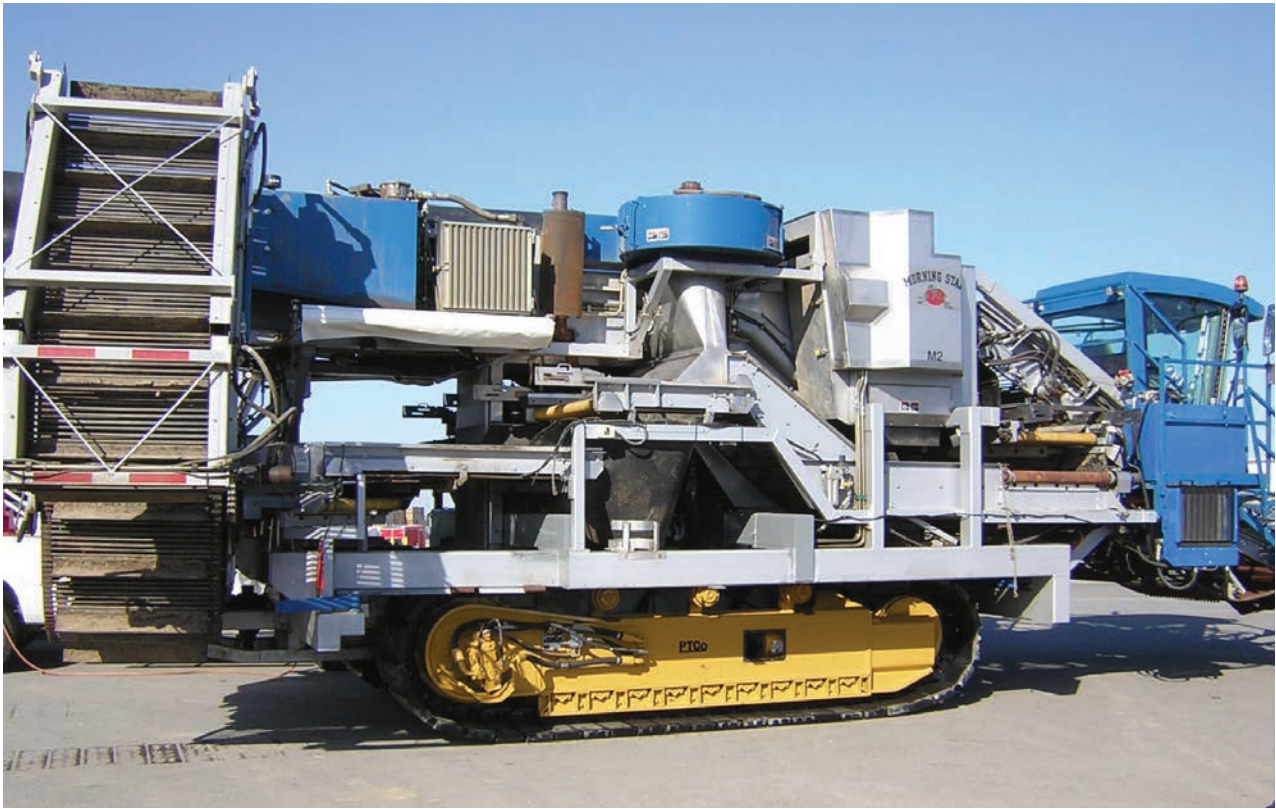
Tomato Harvester with custom-built undercarriage
