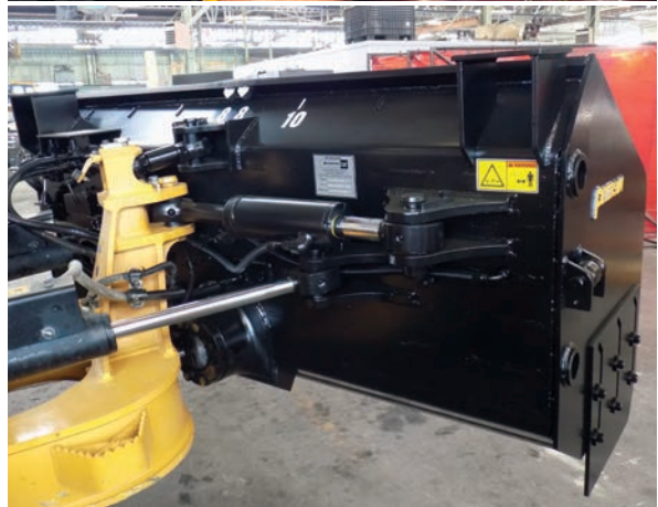
Engineer Dale Smith built the telescoping 7-way blade with AutoCAD software before it was built in the San Leandro fab shop.
